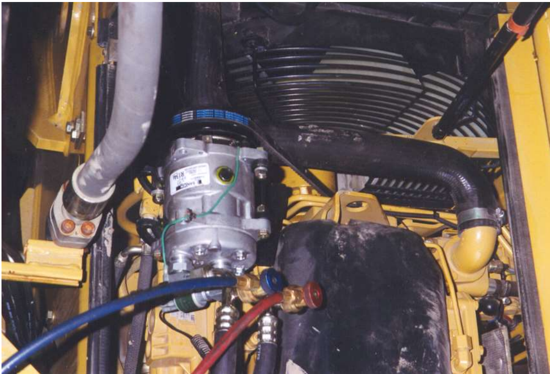
Compressor location on engine with hoses in place.
