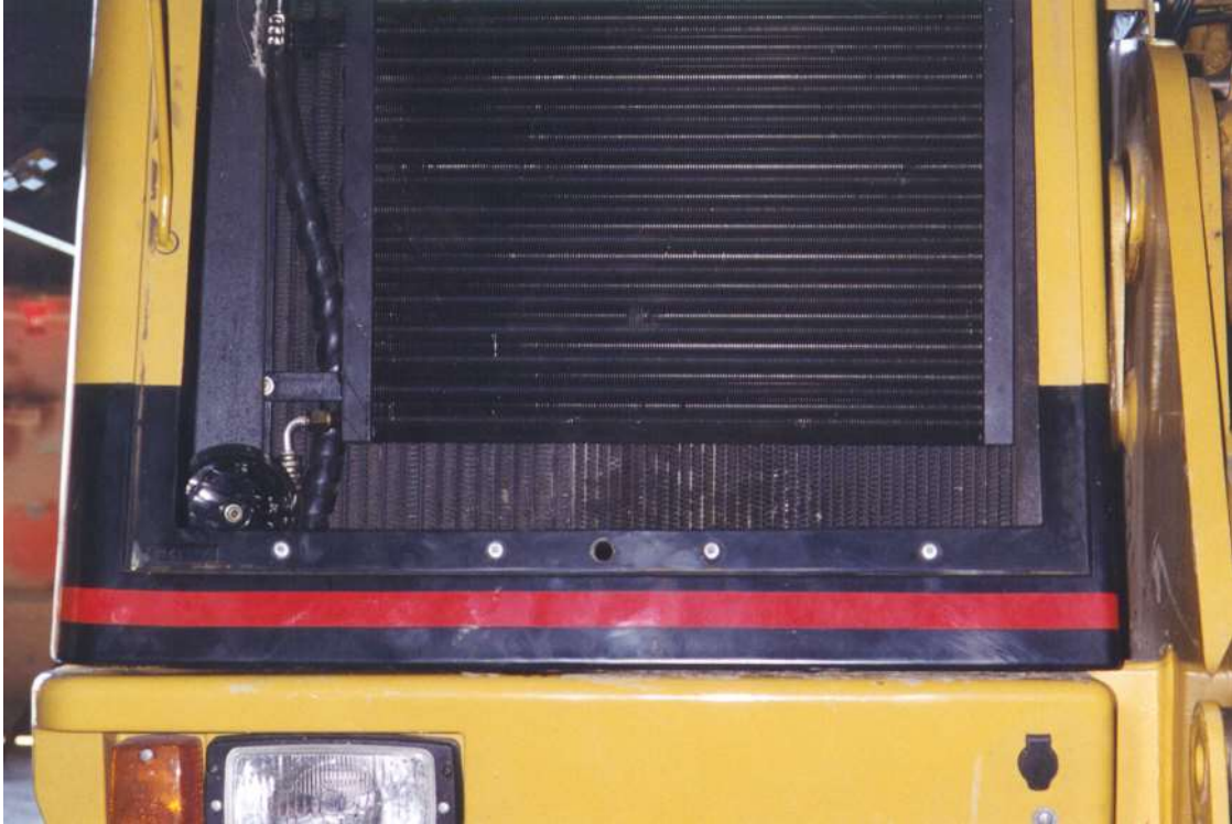
Condenser in place with radiator cowling installed.
