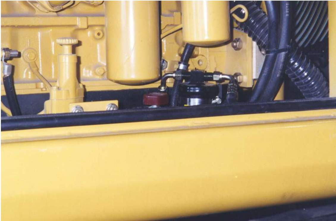
Drier in place alongside engine.
