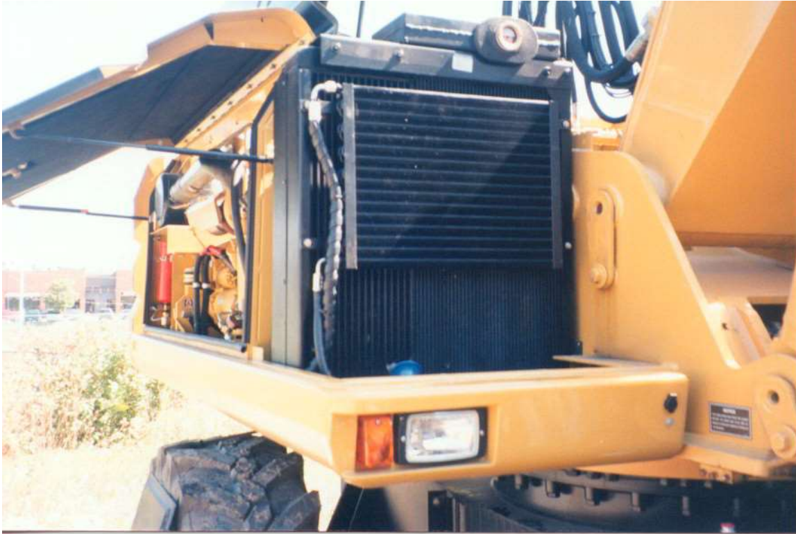
Condenser in place on frame with radiator cowling removed.
